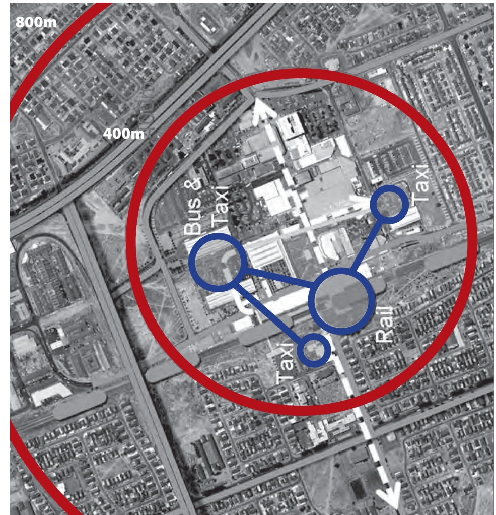
Figure 9: Aerial photograph of Mitchell's Plain town centre, showing application of the Interchange Zone concept
